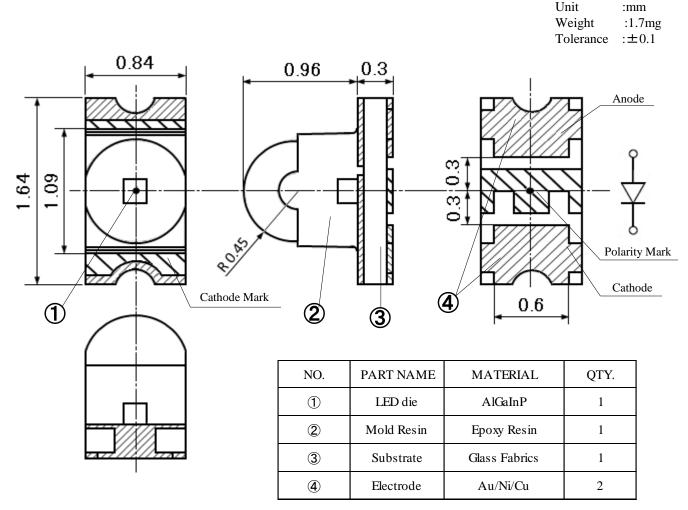
Note : The cutting burr of the substrate and electrodes doesn't contain size of the product.
