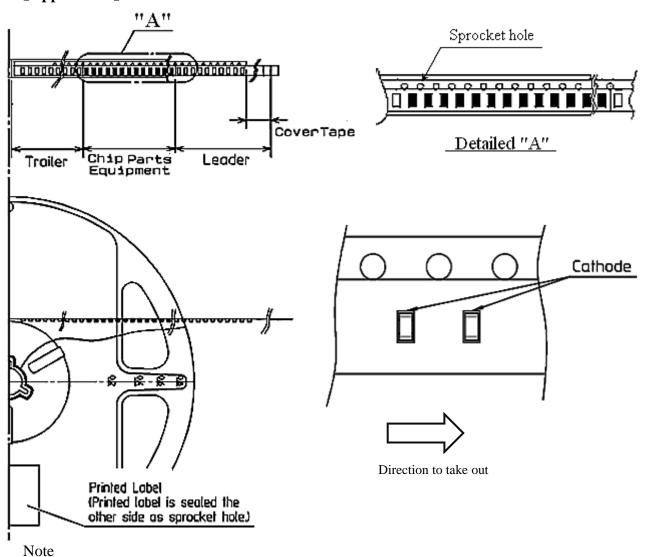
"-TR" means Cathode Side of LEDs should be placed on the sprocket-hole side.
