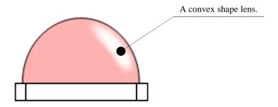
Please adjust the load, the pick up point, the nozzle diameter and etc. before mounting because the over load can cause the breakage of the surrounding of LED.
