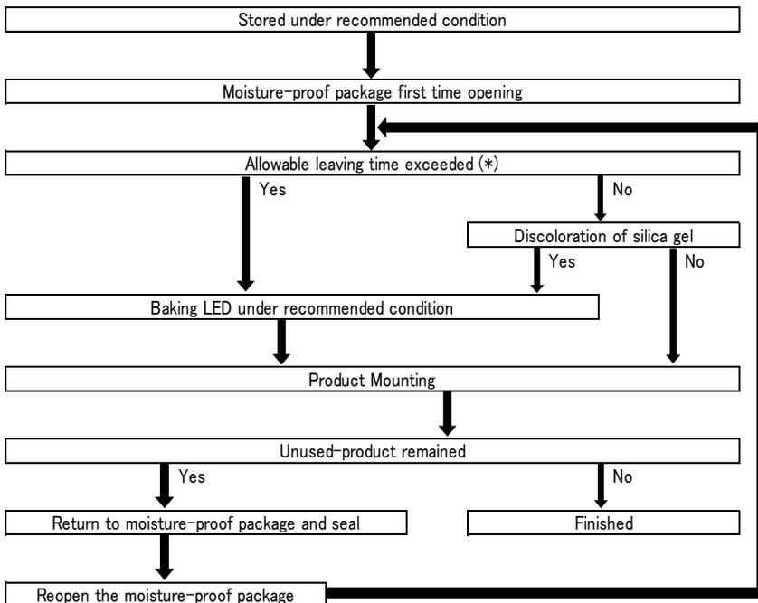
Allowable leaving time means the maximum allowable leaving time after opening package, which depends on each LED type. The allowable leaving time should be calculated from the first opening of package to the time when soldering process is finished. When judging if the allowable leaving time has exceeded or not, please subtract the soldering time after reopening should be calculated from the first opening of package, or from the time when baking process is finished.
