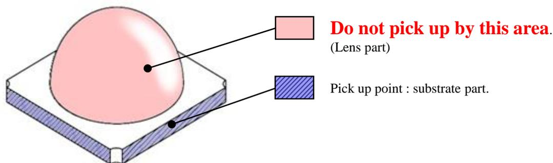
13. Please avoid overload to the product when using tweezers to pick up LEDs.
