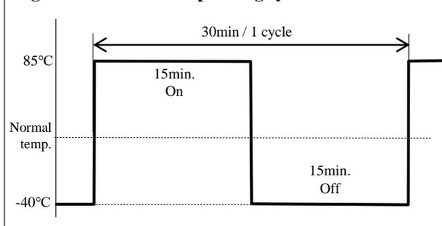
**Fig.2 Thermal & high temp. cycle test condition**
