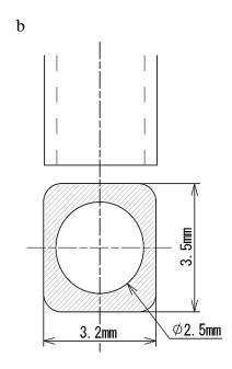
\*Nozzle with chamfering is recommended
