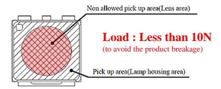
Please adjust the load, the pick up point, the nozzle diameter, etc. before mounting because the over load can cause breakage of the lamp housing.
