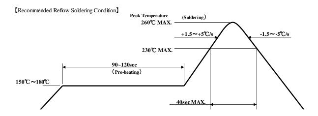
Note 1 Recommended temperature profile for the reflow soldering is listed as the temperature of the resin surface. This should be the maximum temperature for soldering. Lowering the heating temperature and decreasing heating time is very effective in achieving higher reliability.
