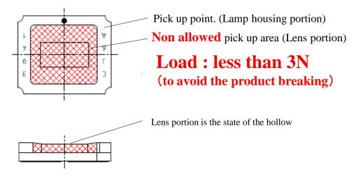
Please adjust the load, the pick up point, the nozzle diameter, etc. before mounting because the over load can cause the breakage of the lamp housing.
