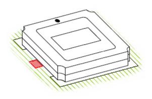
Recommended solder temp. measurement point
