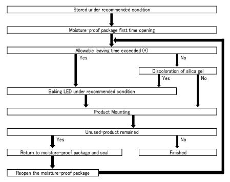
Allowable leaving time means the maximum allowable leaving time after opening package, which depends on each LED type.
