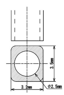
\*Nozzle with chamfering is recommended
