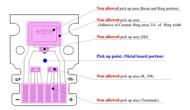
Please adjust the load, the pick up point, the nozzle diameter, etc. before mounting because the over load can cause the breakage of the lamp housing.
