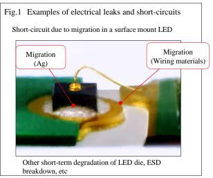
Electrical leaks and short-circuits are caused either by faults or degradation in the semiconducting properties of the LED die, or by electrochemical changes in the materials used.
