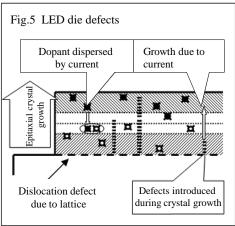
However, there are in fact a number of factors that impede this process, the primary problems being intracrystalline defects and the presence of impurities.
