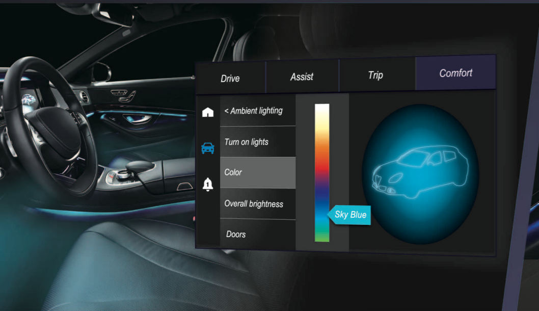
Shy Tech display Hidden beneath textiles or plastics, visible when switched-on
