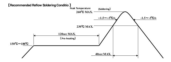
Note 1 Temperature Profile for the reflow should be set to the surface temperature of resin which is on the top of Photo detector. This should be the maximum temperature for soldering. Lowering the heating temperature and decreasing heating time is very effective in achieving higher reliability.
