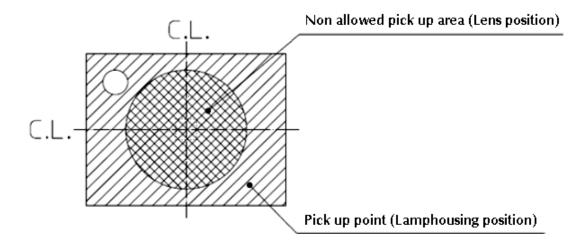
Please adjust the load, the pick up point, the nozzle diameter, etc. before mounting because the over load can cause the breakage of the lamp housing.
