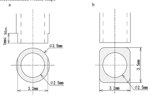
Nozzle with chamfering is recommended
