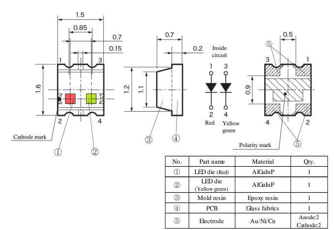
Note : The cutting burr size of the substrate and pin isn't contained in the size of the height of the product.
